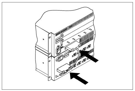
Figure 8. Attaching the Expansion Interface Cable
